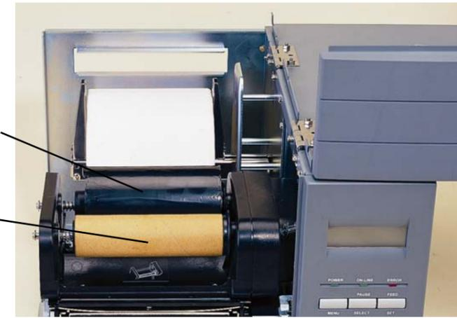
4. Open the printer cover and install the label roll
