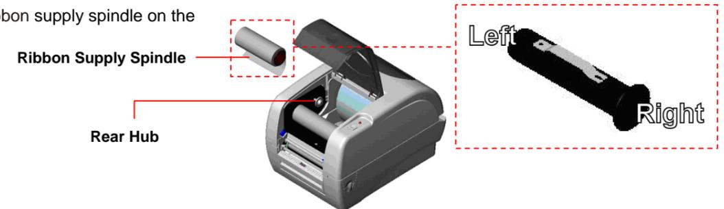
6. Open the printer's top cover by releasing the green top cover open levers located on each side of the printer and lifting the top cover. Pull the ribbon from the ribbon supply spindle and cross the print head, stick the ribbon onto the ribbon rewind paper core.
