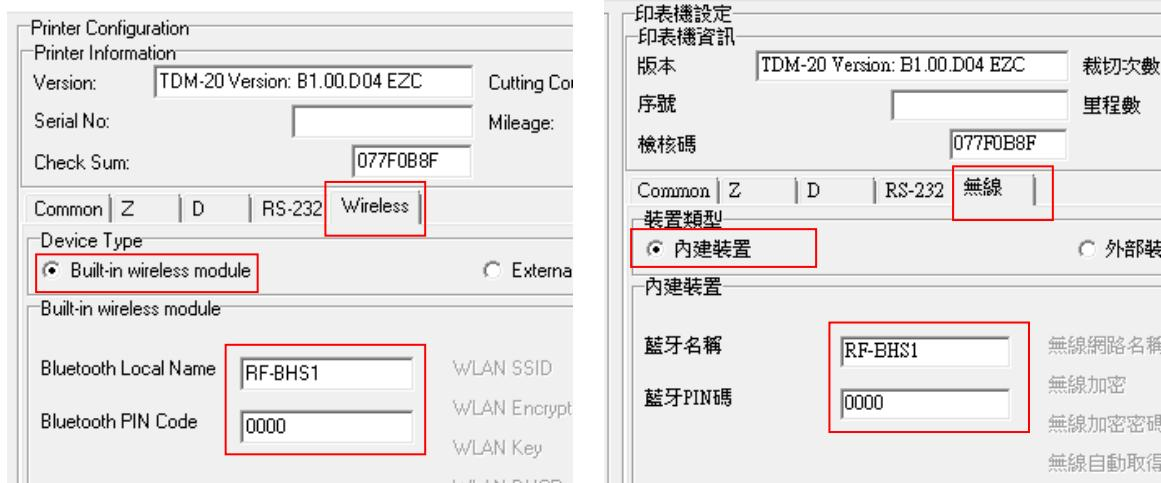
5. Press "Set" button to set the new BT name or BT PIN code of the printer.
